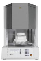
Due to the size of the heating chamber, it is now possible to process three sintering trays  $\emptyset$ <sub>=</sub> 120mm during the conventional long-term sintering. However, the heating system with six high-quality molybdenum disilicide heating elements (MoSi2) enable you to carry out processes within 76 minutes in a SPEED-sintering process. These represent optimal prerequisites for your dental laboratory or milling centre.
